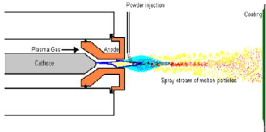
Fig. 1. Schematic Diagram of the Plasma Spray Process.
